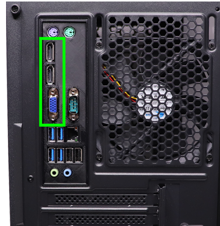
Figure 1: Connection if no graphics card
